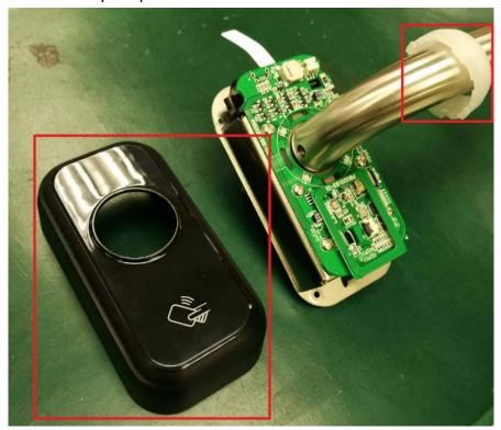
3. Loosen the screw of handle and change the handle direction
